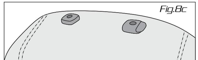
Once complete, refit cover as noted in Steps 3-6 and tuck the cut headrest holes under the plastic trimming (Fig. 8c).
